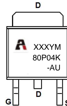
Marking and pin assignment
