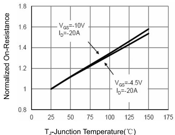
**Figure 8 Drain-Source On-Resistance**
