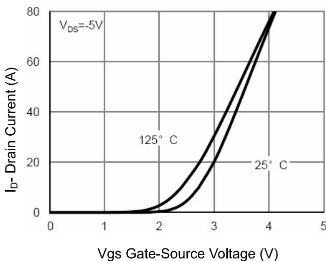
**Figure 7 Transfer Characteristics**
