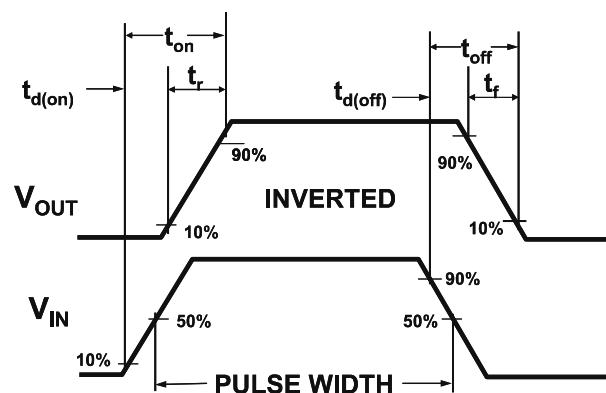
Figure 2 Switching Waveforms
