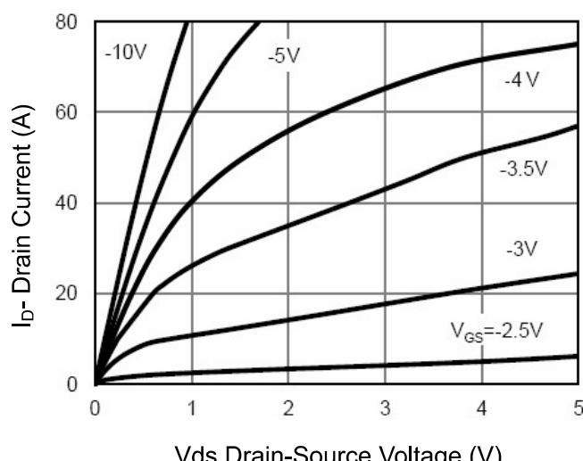
Figure 5 Output Characteristics
