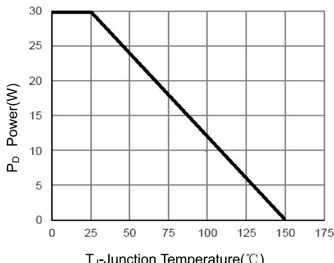
Figure 3 Power Dissipation
