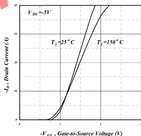
Fig 11. Transfer Characteristics
